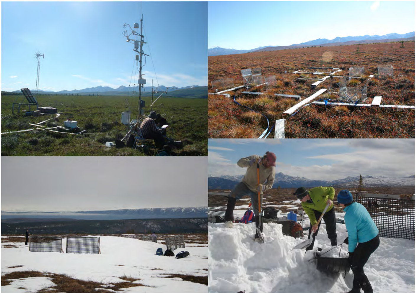
Figure 2. Clockwise from top left: A) Eddy covariance tower measuring landscape carbon dioxide and methane fluxes at the Permafrost Thaw Gradient; B) CiPEHR and DryPEHR with carbon dioxide flux chambers and air warming chambers during the growing season; C) CiPEHR in winter with snow fence and drifted snow passively warming soils and thawing permafrost; D) snow removal occurs in spring to maintain constant water inputs and constant spring melt date between warming and control plots. Images courtesy of Maurtiz and Schuur.
