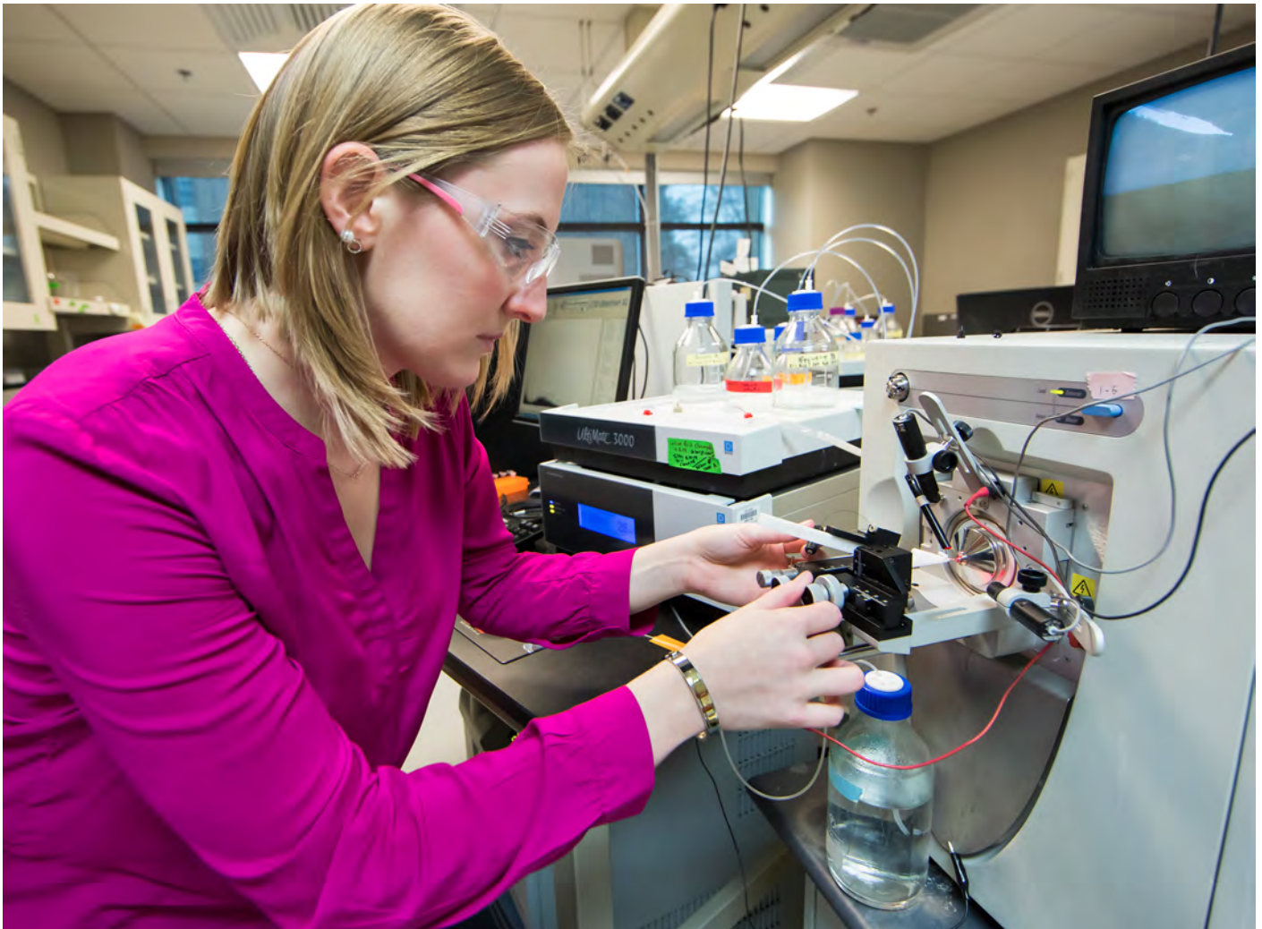
Mallory Ladd uses liquid chromatography and high-resolution mass spectrometry to characterize the molecular composition of nitrogen in soil samples from a polygonal tundra near Barrow, Alaska. Photo courtesy of Joy Anderson, ORNL.
