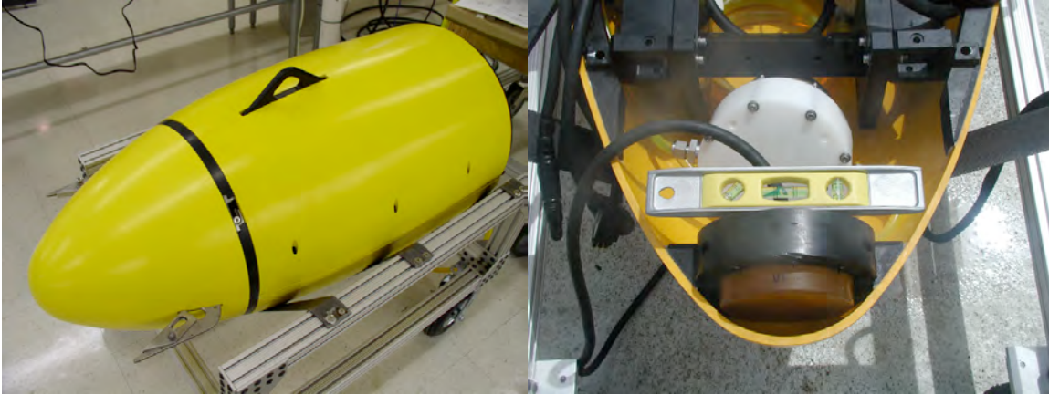
Figure 5. Nose cone detail of APOGEE AUV, and AUV specifically designed for under-ice operation. Left panel shows nose cone with side hooks for latching to a trawl wire suspended from an icebreaker or hole in the ice. Right panel shows acoustic homing transducer inside nose cone that allows the vehicle to determine the azimuth and bearing of an acoustic beacon affixed to a trawl wire for vehicle recovery through the ice.
