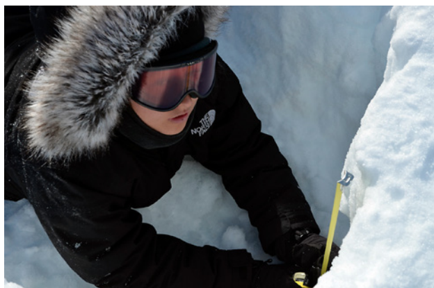
Student participant Nivi Rosing of Nuuk, Greenland, measures depth of fluid penetration into ice during an experiment at NEEM. Photo courtesy of Peter West.
